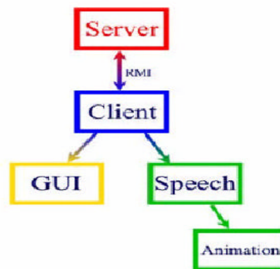
Figure 1. A simple overview of the communication system from the client perspective
